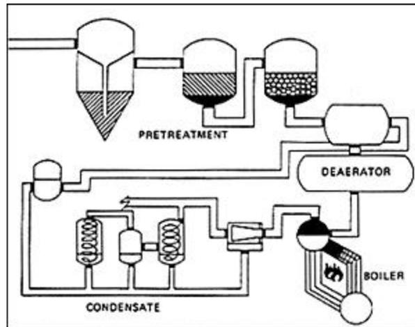
The purpose of a boiler is to produce steam for heating, for plant processes, and for driving turbines that produce electricity. While boiler systems vary in shape and size, they typically consist of the Boiler and its support systems: Pretreatment, Condensate, and Feedwater.
