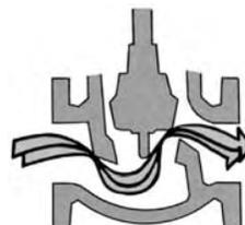
Globe valves are used to throttle efficiently. Seating is parallel to the lone of flow. The change in direction of fluid flow through these valves produces increased resistance and considerable pressure drop.
