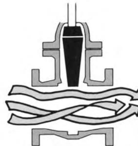
Gate valves are used where it is important that pressure drop through the valve is minimal.
