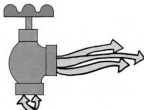
Angle valves have the same features of stem, disc and seat ring design as the globe valve. The fundamental difference between the two is that the fluid flow through the angle valve makes a 90° turn. These valves offer less resistance to flow than a globe valve with an elbow which it would replace. An angle valve reduces the number
