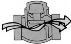
Special ball check valves are available for slurry applications.
