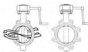
When selecting larger throttling valves using flanged piping connections, butterfly valves should be considered.
