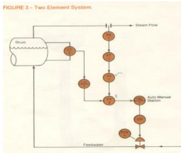
*Two-Element Control, drawing courtesy of Honeywell*
